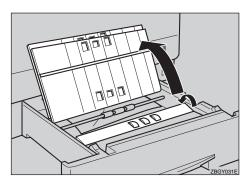
Remove the misfed paper under the guide while closing towards you as shown in the illustration.
